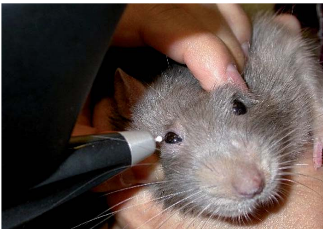
Fig. 3 The Rebound Tonometer is invaluable for measuring intraocular pressure in the small eyes of rodents.
